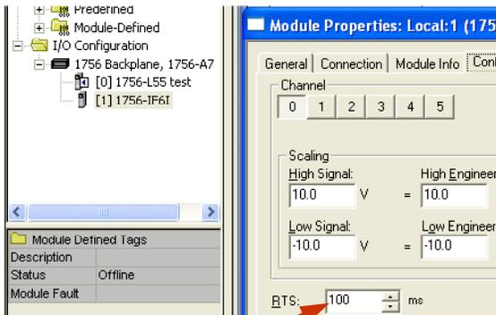
Configure the analog input module for your desired RTS rate.
